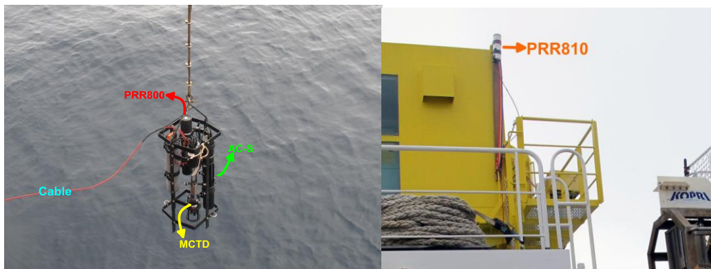
Figure .6.6.The left figure shows the frame designed for deploying PRR800, ACS and MCTD; The right one shows PRR810 at the top of yellow crane
