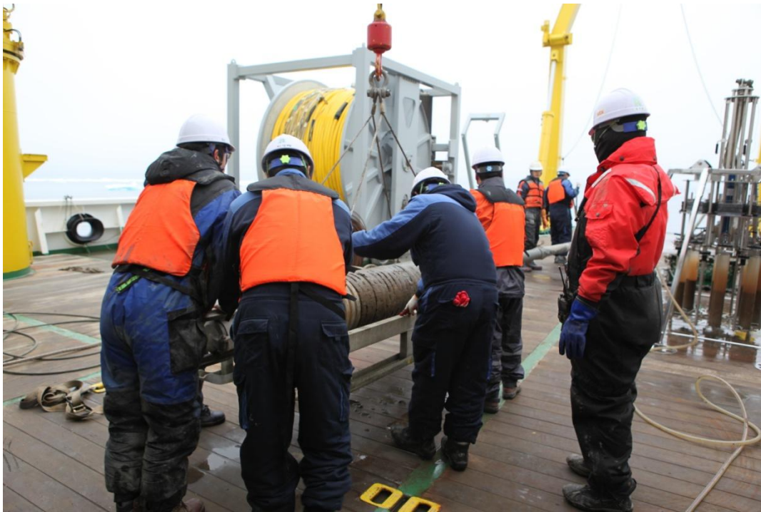
Figure 7.14 Long sediment cores are recovered with a gravity corer
