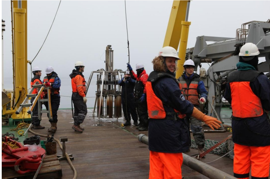
Figure 7.13 Surface sediment with overlying bottom water were taken with multiple corers
